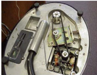
Figure 11. Series A –T Blender drive system with tensioner.
