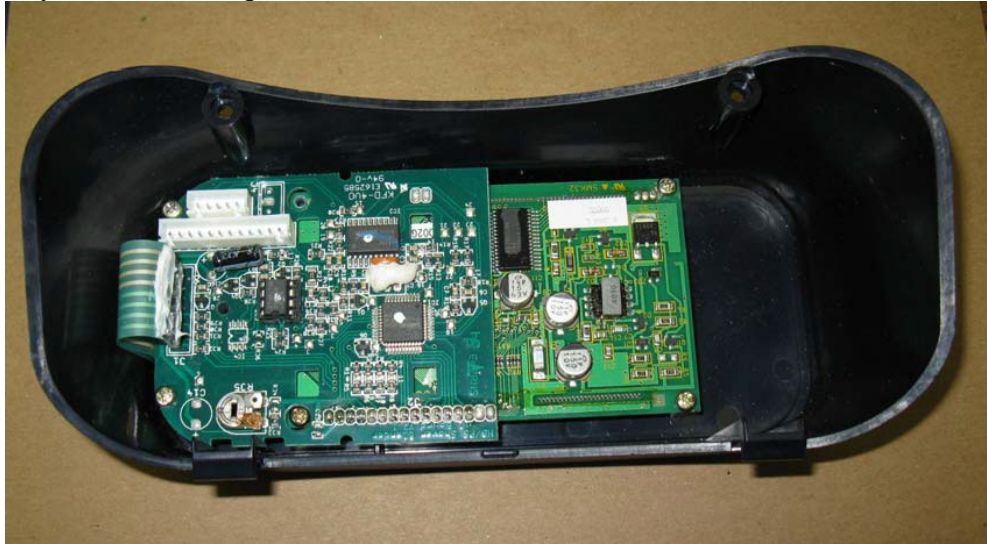
Fig. 21. Rear of Control Panel removed from unit.
