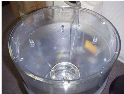
Figure 2. Fin orientation in the front of the machine.
