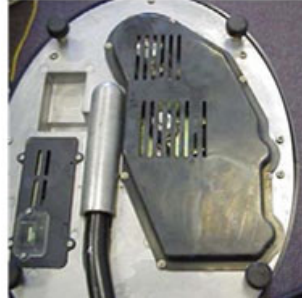
Figure 10. Cover over blender drive system.
